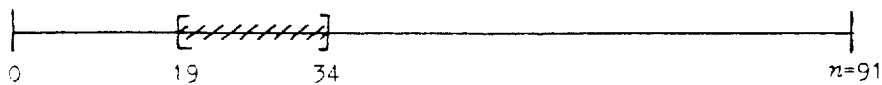
Fig. 2. The valid messages with left-padded redundancy for n=91 , l=19 and u=34 . The valid messages are 19, 20, 21, ..., 34. The actual messages are 0, 1, 2, ..., 15.
